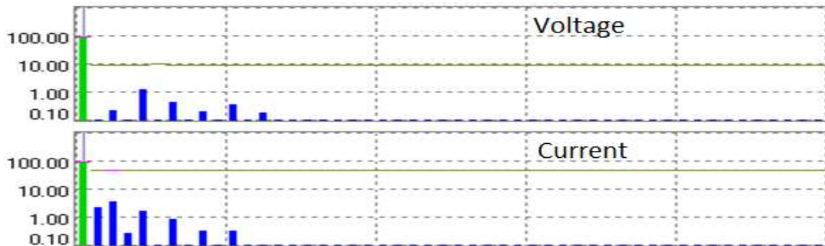
Fig. 12 Voltage and current harmonic spectrum for Compressor
