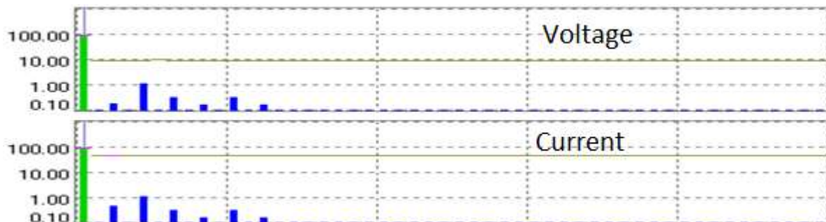
Fig. 9 Voltage and current harmonic spectrum for incandescent Lamp
