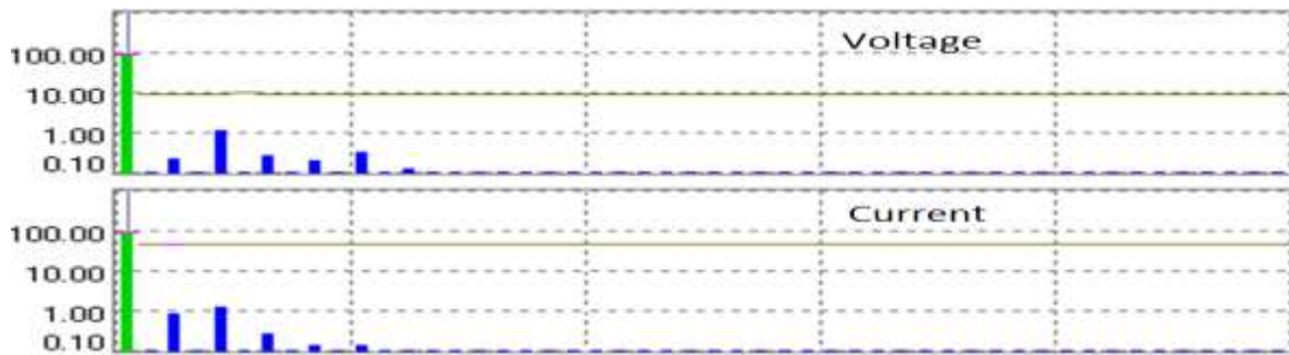
Fig. 21 Voltage and current harmonic spectrum for Fan
