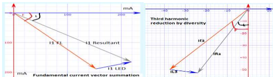
Fig. 26 Fundamental current displacement angle improvement and third harmonic reduction due to diversity
